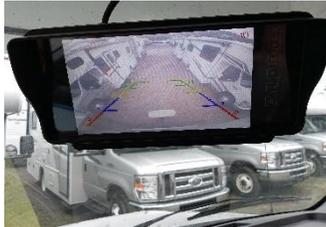
The RV is equipped with a backup camera and blind spot cameras in your side mirrors. The back up camera will come on when you shift into the reverse gear. As well you can see your blind spots when you use your turn signals.
