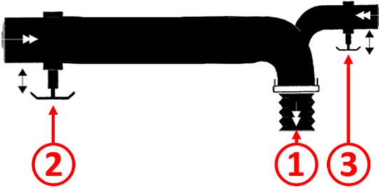
1. Remove cap from the sewer outlet ①.
