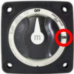
The main switch for turning the coach batteries on and off is located directly next to the side entrance door at floor level. This switch must be in the **ON** position to supply 12-volt power to the appliances and living area. When there is no power in the living area, always check to see if this switch may have been set to OFF accidentally and reset to ON if necessary.
