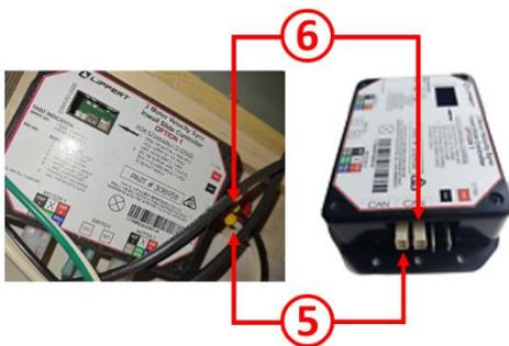
If the reset does not have the desired result, first disconnect the white cable **⑤** (power connection) from the module and wait for 30 seconds before reconnecting it. Repeat this step with the ground cable **⑥** (red or black). Now try to operate the slide-out. If this procedure does not help retract the slide-out, the problem may be due to moisture in the slide-out module. Try eliminating the moisture using a hairdryer (only in dry weather!) and then repeat the above steps.
